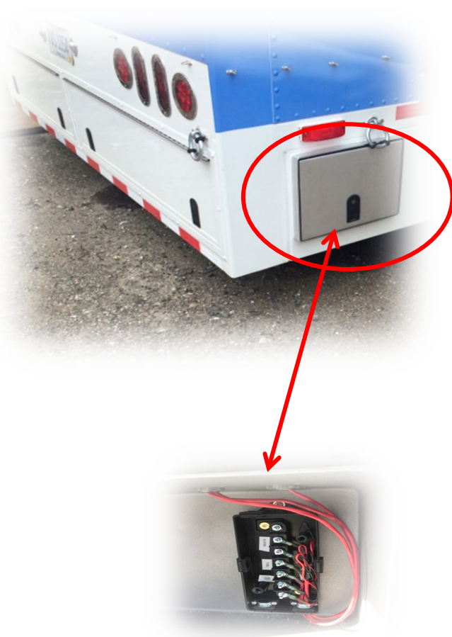
Fire Alarm Connection Customer Connection Point Fire Alarm Remote Dry Contacts
