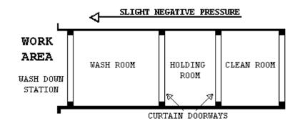
F. Waste/Equipment Decontamination Procedures: At the washdown station in the regulated area, thoroughly wet wipe/clean contaminated equipment and/or sealed polyethylene bags and pass into Wash Room after visual inspection. When passing anything into the Wash Room, close all doorways of the W/EDF, other than the doorway between the washdown
