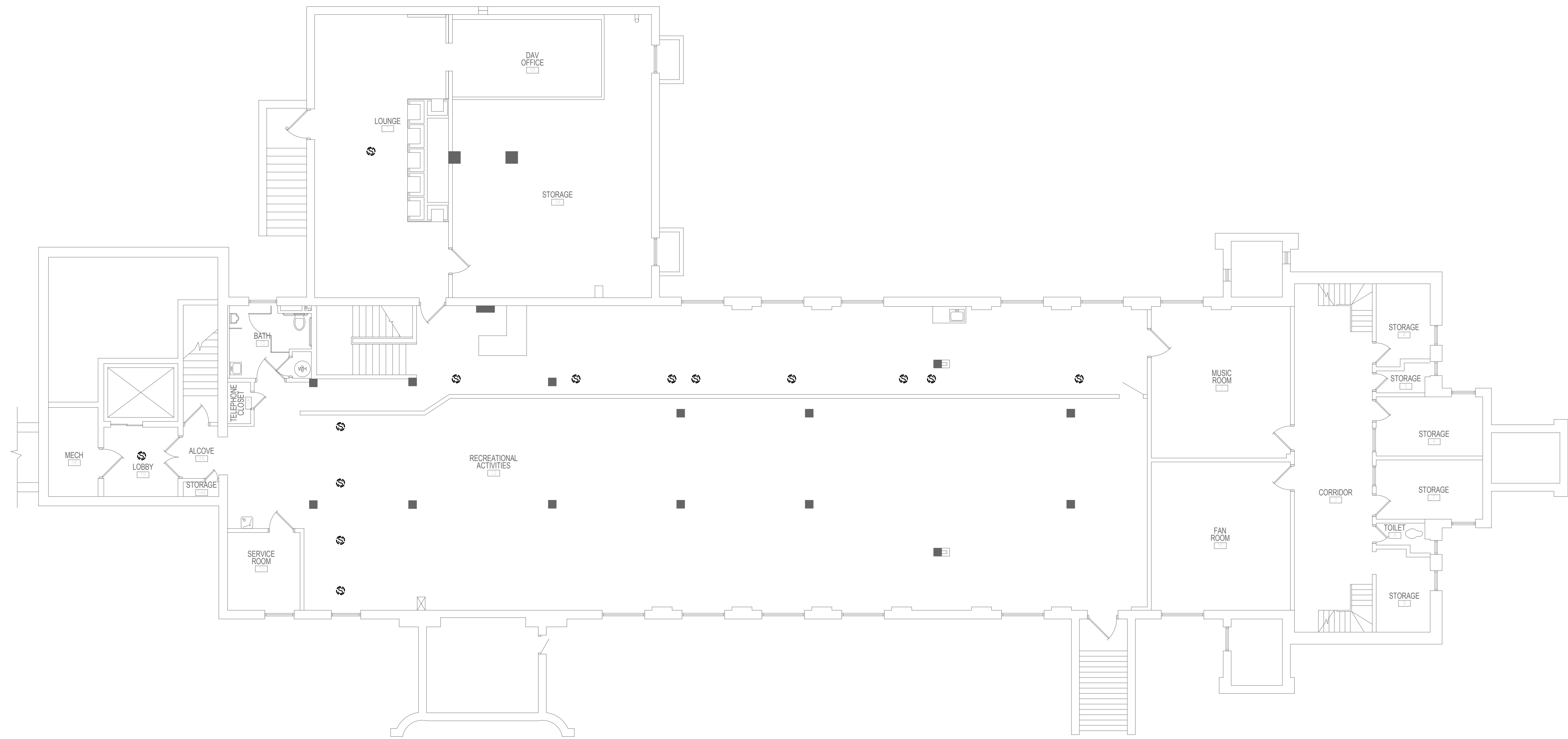
1 BUILDING 08 - PAGING SPEAKER DEMOLITION FLOOR PLAN - BASEMENT 1/8" = 1'-0"
