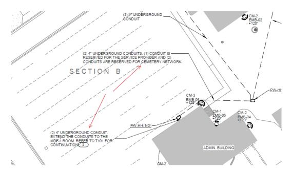
7. On Sheet T100, Would it be acceptable to bore the conduits in between the two maintenance buildings in lieu of cutting and patching the concrete drive? If boring is acceptable it would not be able to be incased in concrete.
