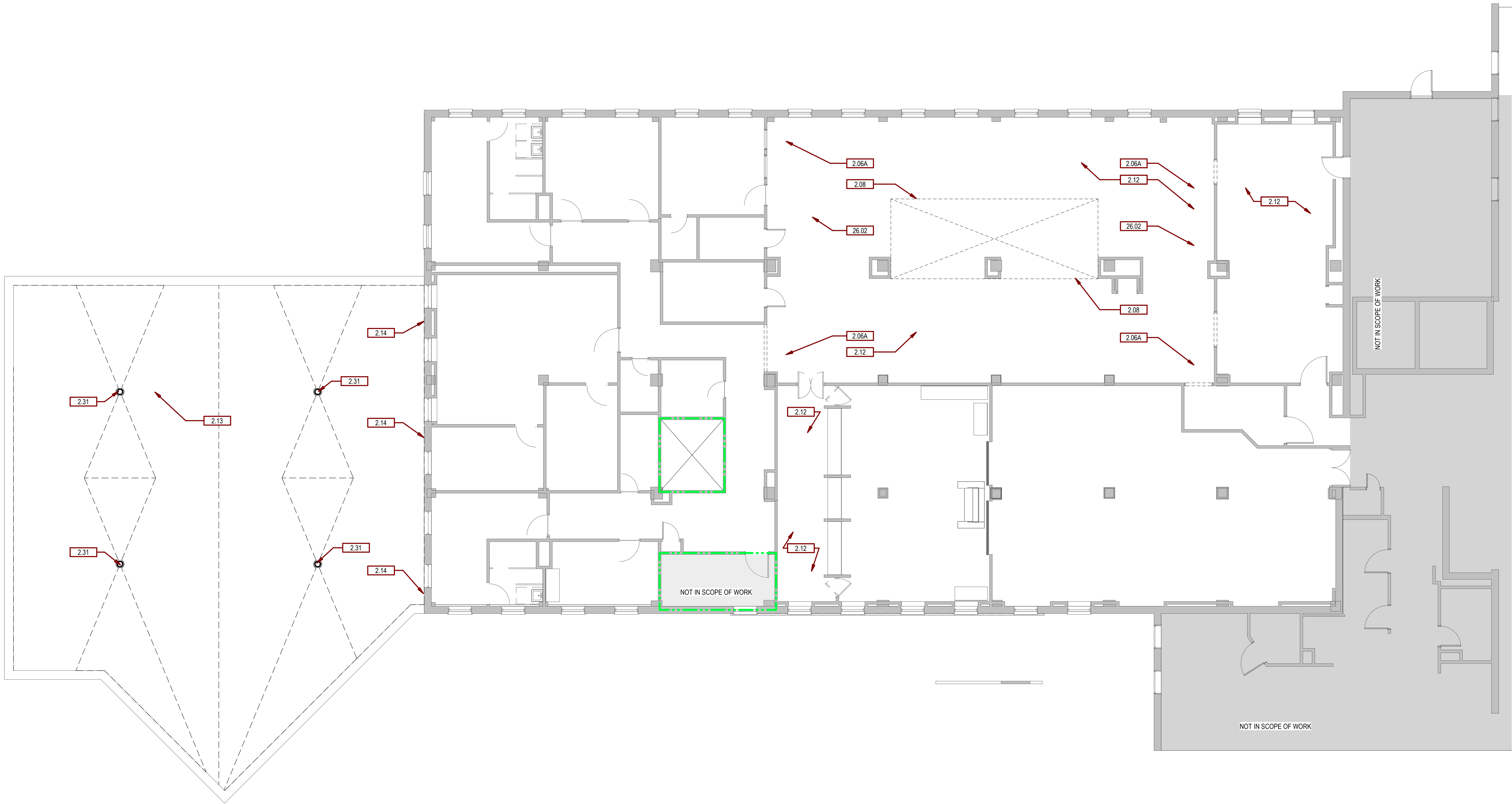
E1 SECOND FLOOR DEMOLITION PLAN 1/8" = 1'-0" NORTH
