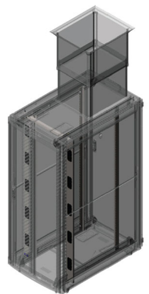
2 ISOMETRIC VIEW WITH DOORS AND VERTICAL EXHAUST DUCT (VED)
