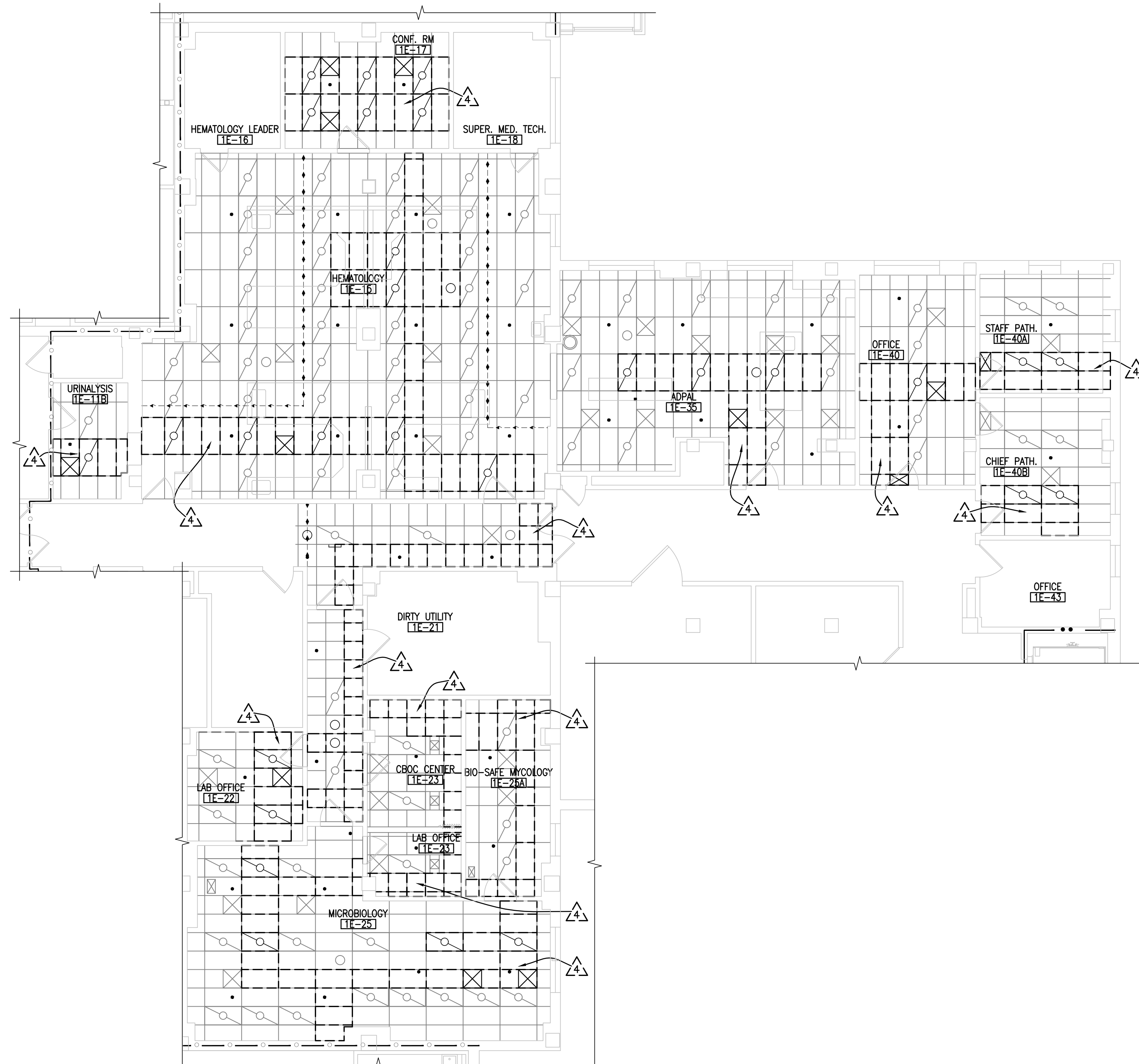
1 PARTIAL FIRST FLOOR - LAB AREA - DEMO RCP SCALE: 1/8" = 1'-0"
