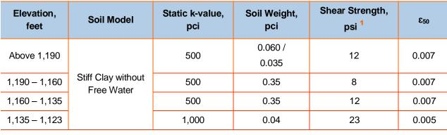
1. The soils encountered in our exploration are cohesive. Therefore, strength is represented by cohesion and not internal friction.
