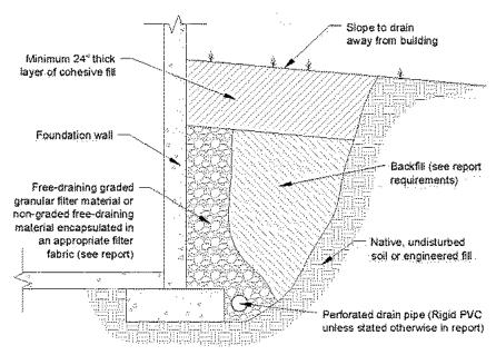
material graded to prevent the intrusion of soil fines into the granular material or the intrusion of the granular material into the drain pipe perforations. Alternatively, a coarse, clean, free-draining granular material could be used to surround the pipe if this material is encapsulated with suitable filter fabric.
