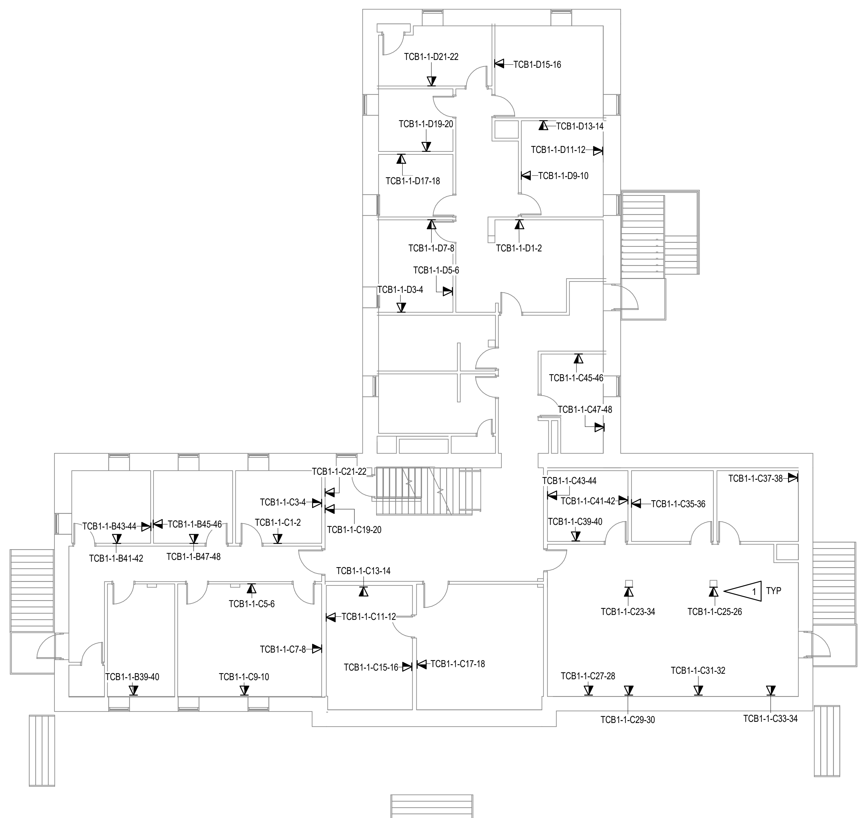
1 TELECOM REMODEL PLAN - BLDG 53 SECOND FLOOR 1/8" = 1'-0"
