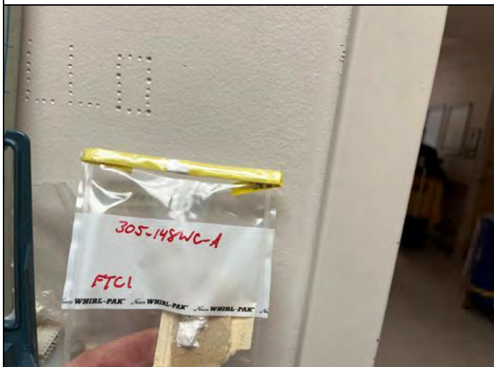
Photo 17 – Sample 305-148WC-A, less than 1% asbestos containing sheetrock and taping compound walls and ceilings in building 148 room FTC1.
