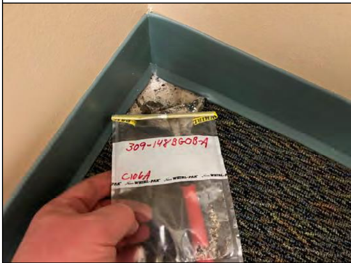
Photo 11 – Sample 309-148T-A, asbestos containing beige over black carpet mastic in building 148, room C106A.
