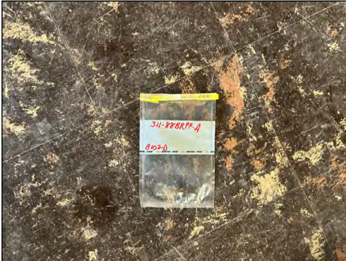
Photo 13 – Sample 311-88BRPP-A, asbestos containing 9" brown w/ pink patches floor tile bldg. 88, room B102D. Tile and mastic contain.
