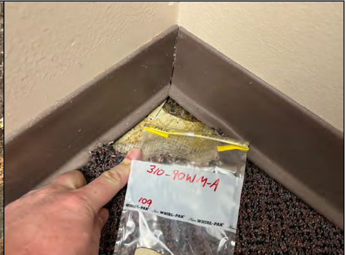
Photo 14 – Sample 310-90WM-A, asbestos containing 12" white mottled floor tile in building 90, room 109. Only mastic contains.
