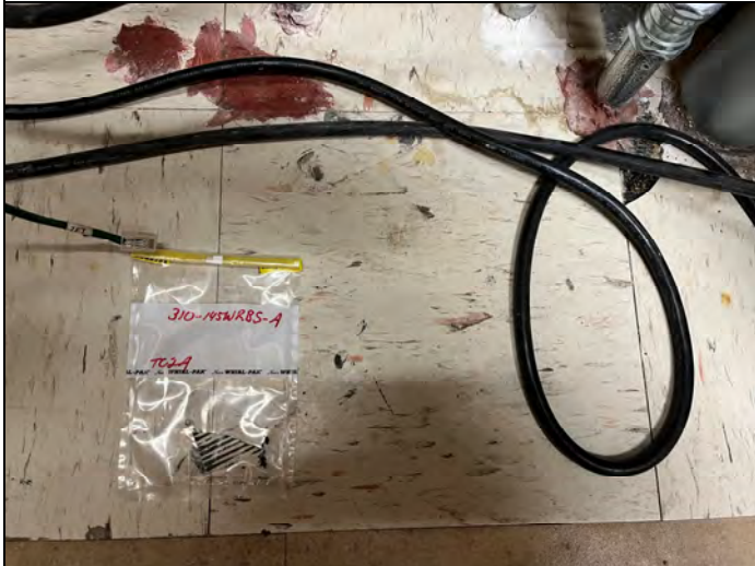
Photo 9 – Sample 310-145WRBS-A, ACM 12" white w/ red and black streaks floor tile in bldg. 145, rm. TC2A. Only mastic contains.
