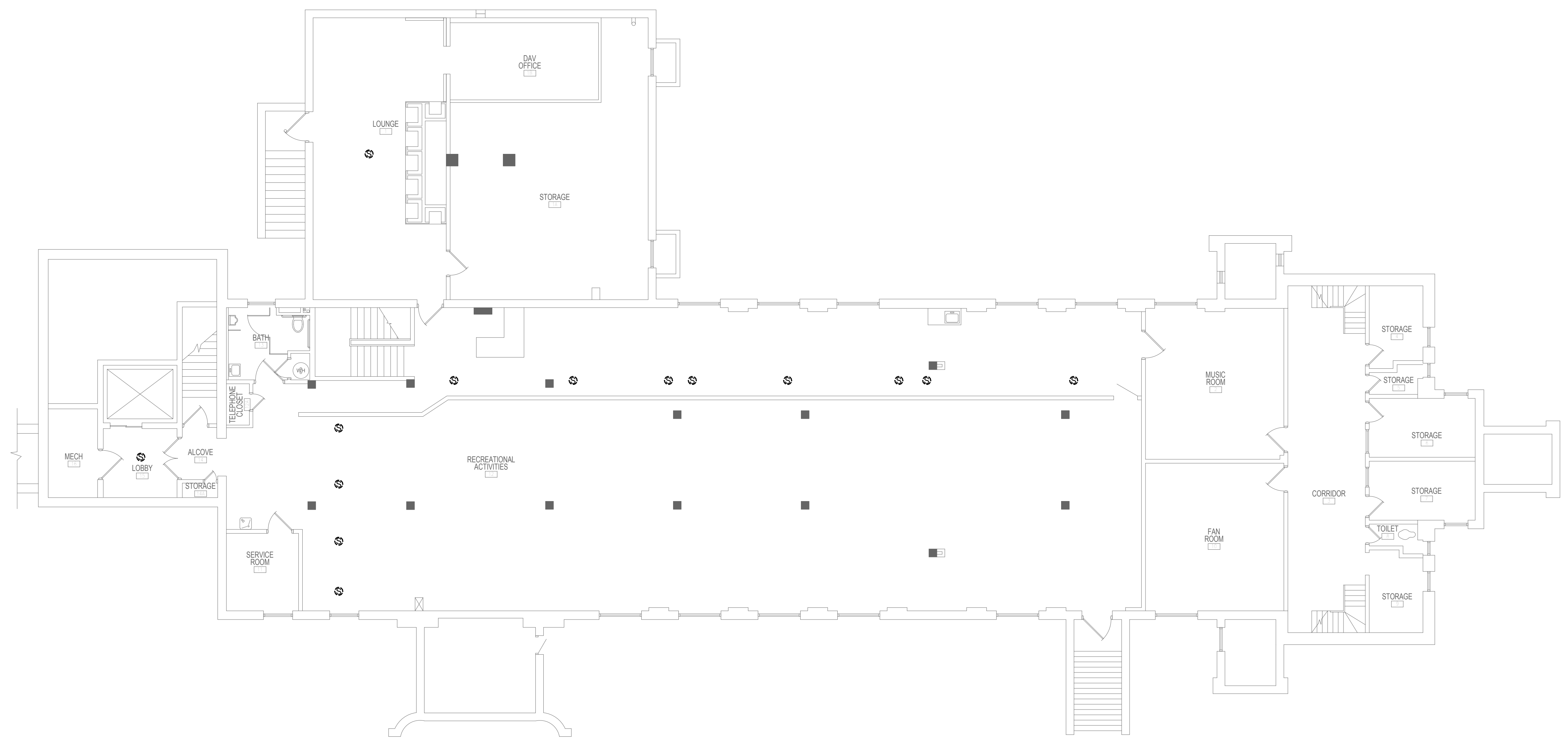
1 BUILDING 08 - PAGING SPEAKER DEMOLITION FLOOR PLAN - BASEMENT 1/8" = 1'-0"
