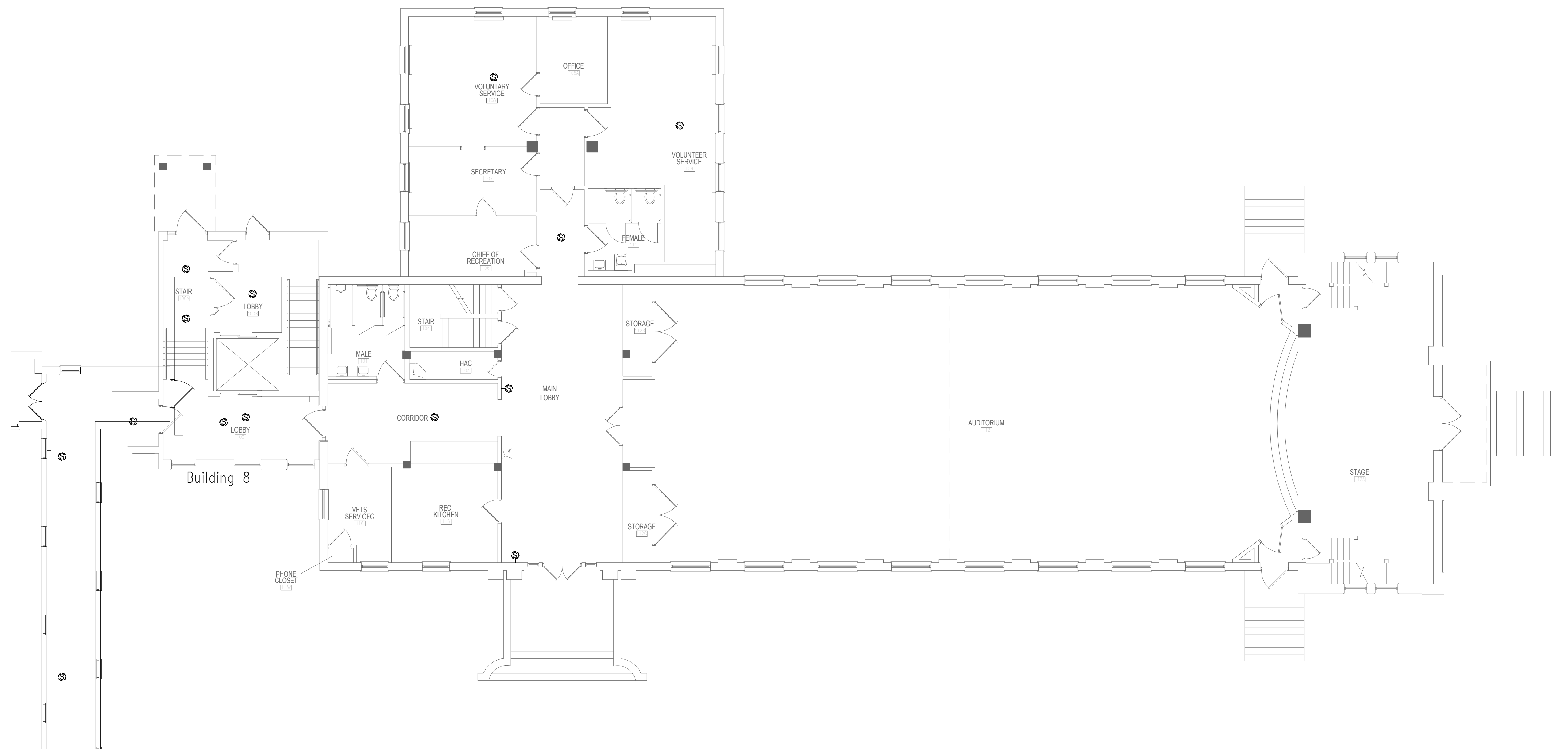
1 BUILDING 08 - PAGING SPEAKER DEMOLITION FLOOR PLAN - FIRST FLOOR 1/8" = 1'-0"
