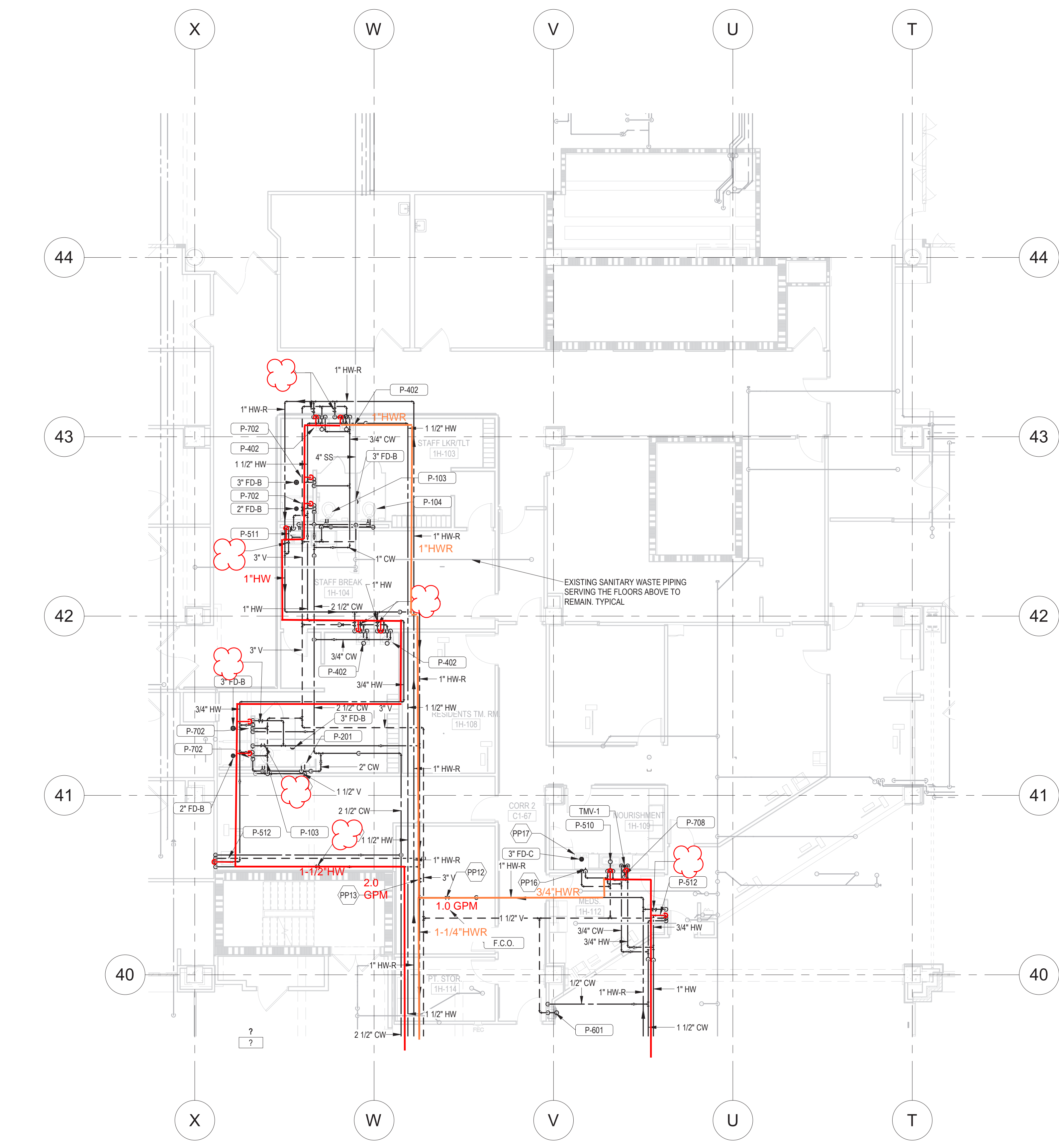
1 LEVEL 1 PLUMBING PLAN, AREA H, PHASE 2 SCALE: 1/8" = 1'-0"
