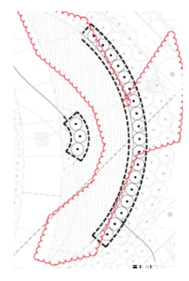
mains. Reinstall new irrigation system outside new sidewalk footprint. Demolish existing irrigation system in areas noted with Red. Install PVC sleeves under new sidewalk for
