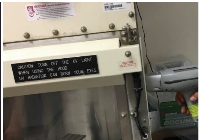
PHOTO 70 Cream Fume Hood – West Wall <1mg/cm 2 lead
