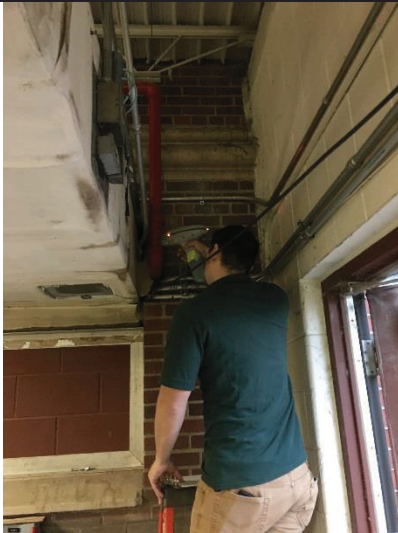
PHOTO 15 Red Painted Pipe – Below Grade Mech. Room <1mg/cm 2 lead
