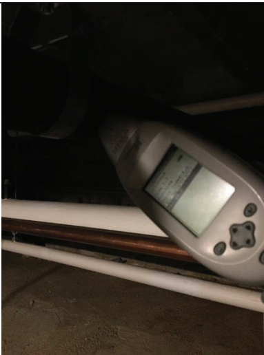
PHOTO 35 Black Pipe – Tunnel <1mg/cm 2 lead
