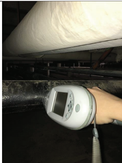
PHOTO 36 Black Pipe – Tunnel <1mg/cm 2 lead
