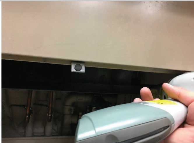
PHOTO 74 Black Metal surrounding sink basin <1mg/cm 2 lead
