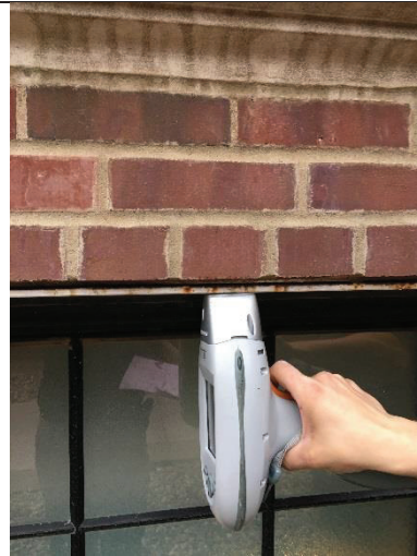
PHOTO 32 White Top Plate – Exterior Window 15 mg/cm 2 lead
