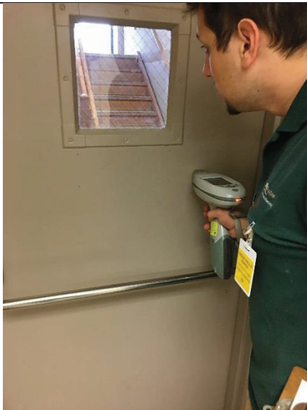
PHOTO 65 Cream Door – S End <1mg/cm 2 lead
