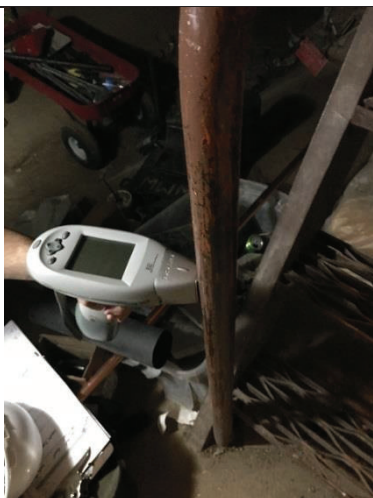
PHOTO 39 Brown Hand Railing-Stairs to Tunnel 3.8\text{ mg}/\text{cm}^2 lead
