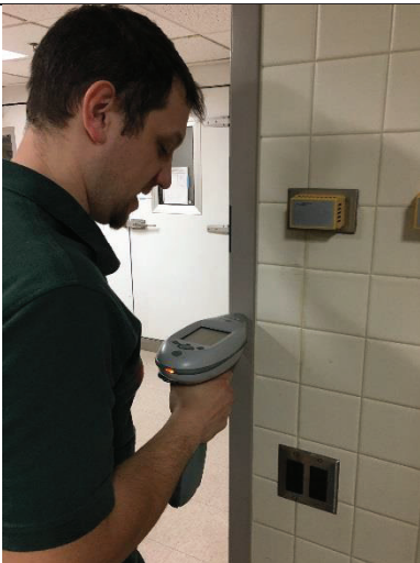
PHOTO 49 Beige Door Frame – D-17 <1mg/cm 2 lead
