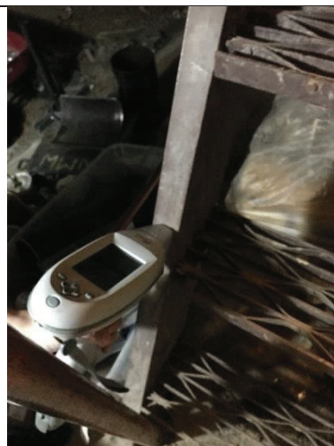
PHOTO 40 Brown Stairs to Tunnel 2.9\text{ mg}/\text{cm}^2 lead
