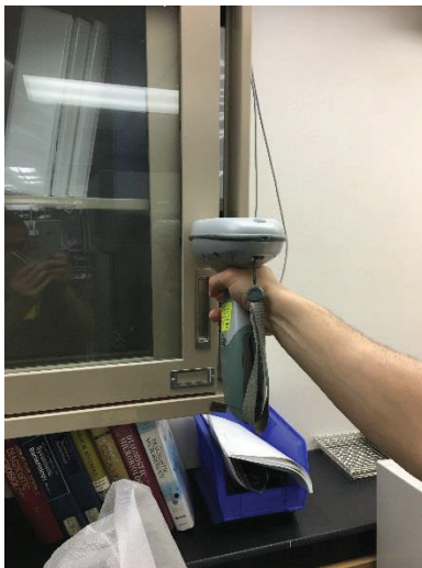
PHOTO 67 Beige Metal Cabinet – S End <1mg/cm 2 lead
