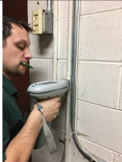
PHOTO 16 White Painted Conduit – Below Grade Mech. Room <1mg/cm 2 lead
