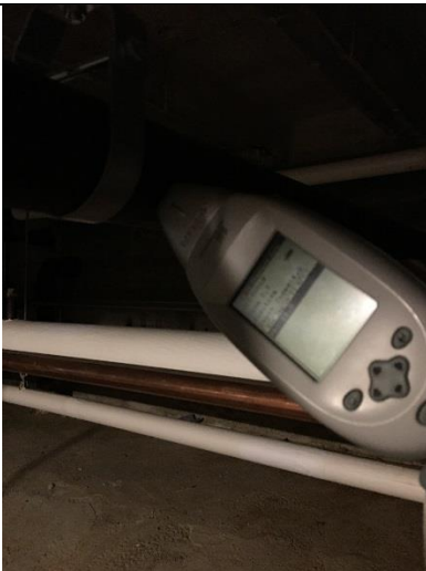
PHOTO 35 Black Pipe – Tunnel <1mg/cm 2 lead
