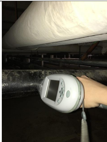
PHOTO 36 Black Pipe – Tunnel <1mg/cm 2 lead
