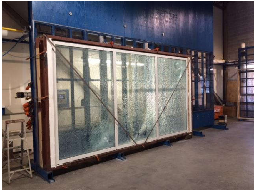
Photo No. 1 Test Specimen After Large and Small Missile Impacts
