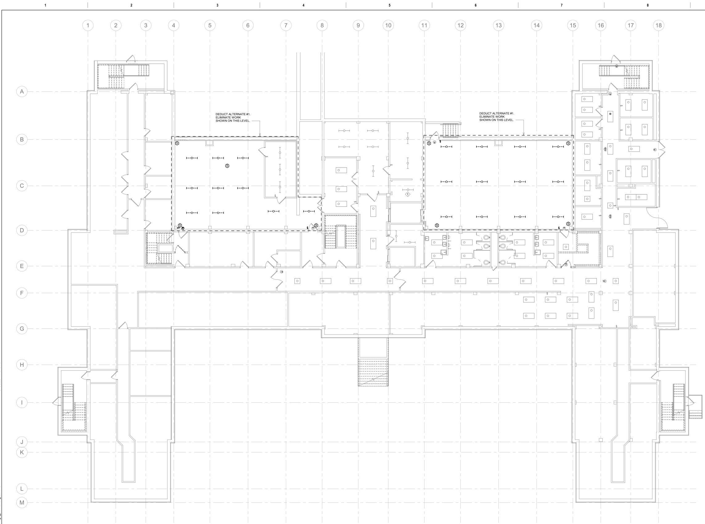
1 BASEMENT LIGHTING DEMOLITION PLAN
