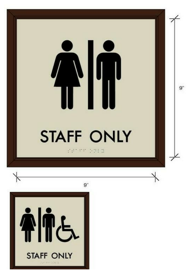
3 SIGN TYPE 99.5 - RESTROOM IDENTIFICATION
