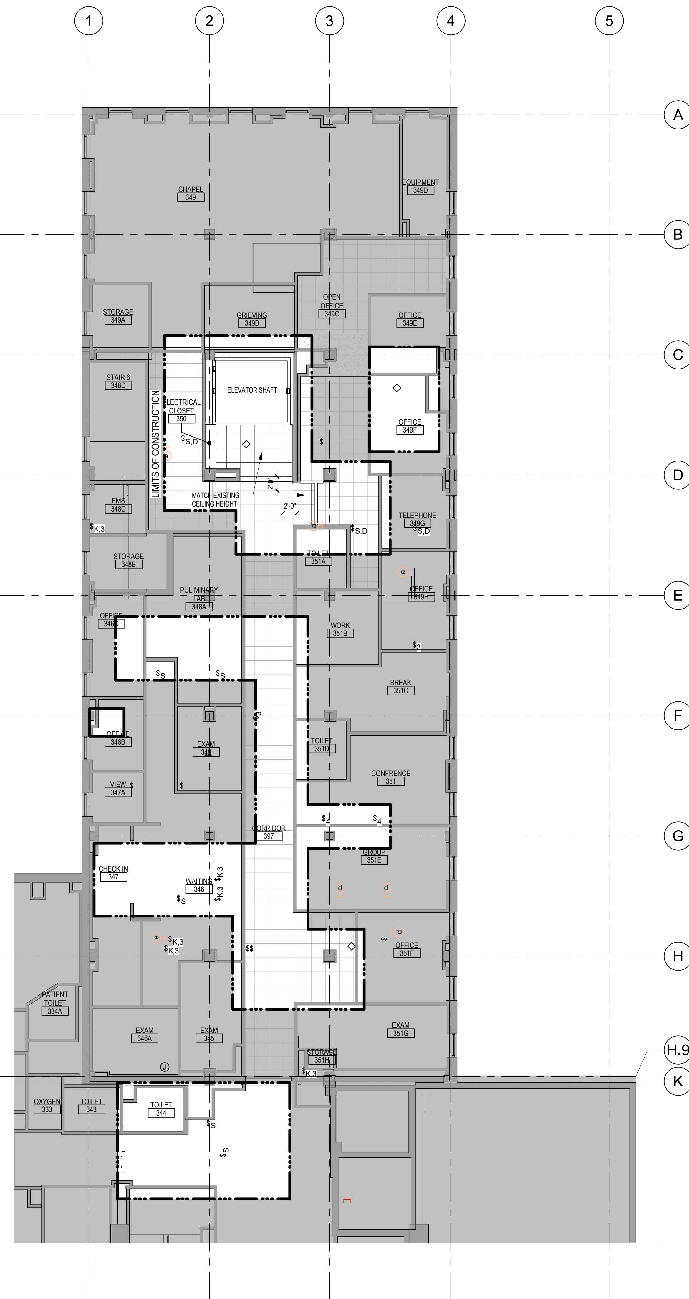
2 THIRD LEVEL REFLECTED CEILING PLAN - BUILDING 5 1/8" = 1'-0"
