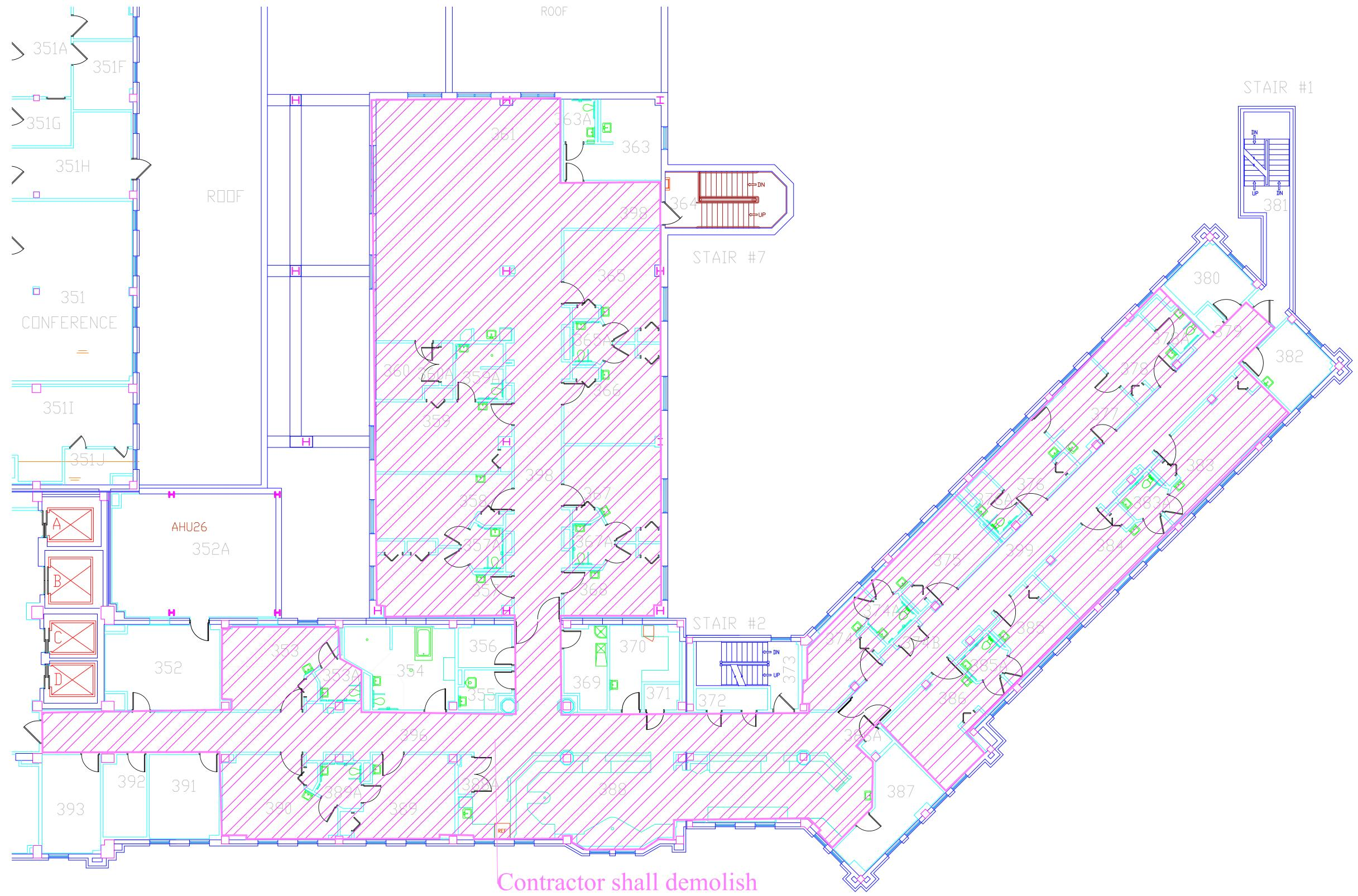
Contractor shall demolish and replace ceiling grid and tile in all areas hatched in pink on plan. See SOW and finish schedule for ceiling grid and tile specifications.
