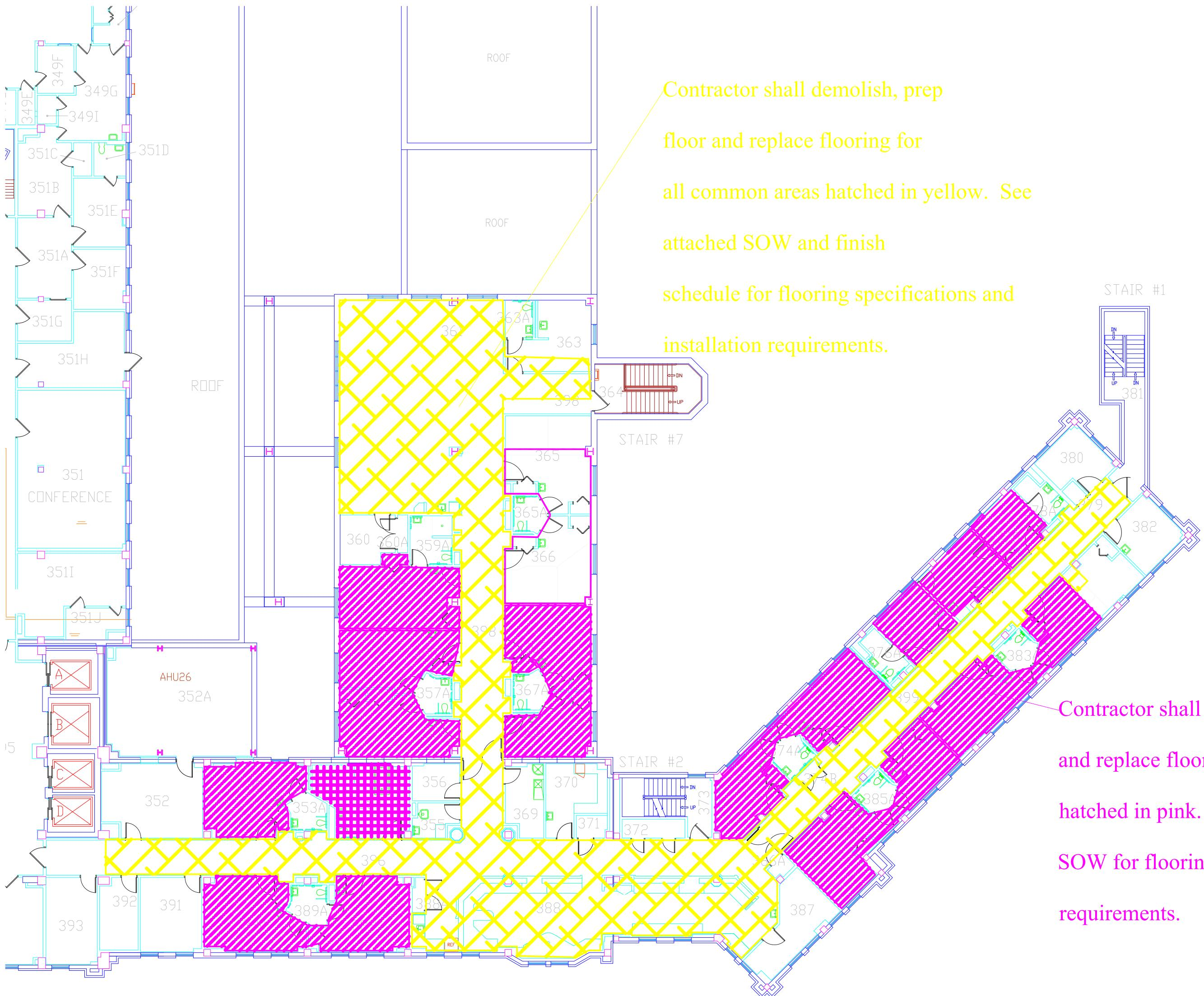
Contractor shall demolish, prep floor, and replace flooring for all inpatient rooms hatched in pink. See attached finish schedule and SOW for flooring specifications and installation
