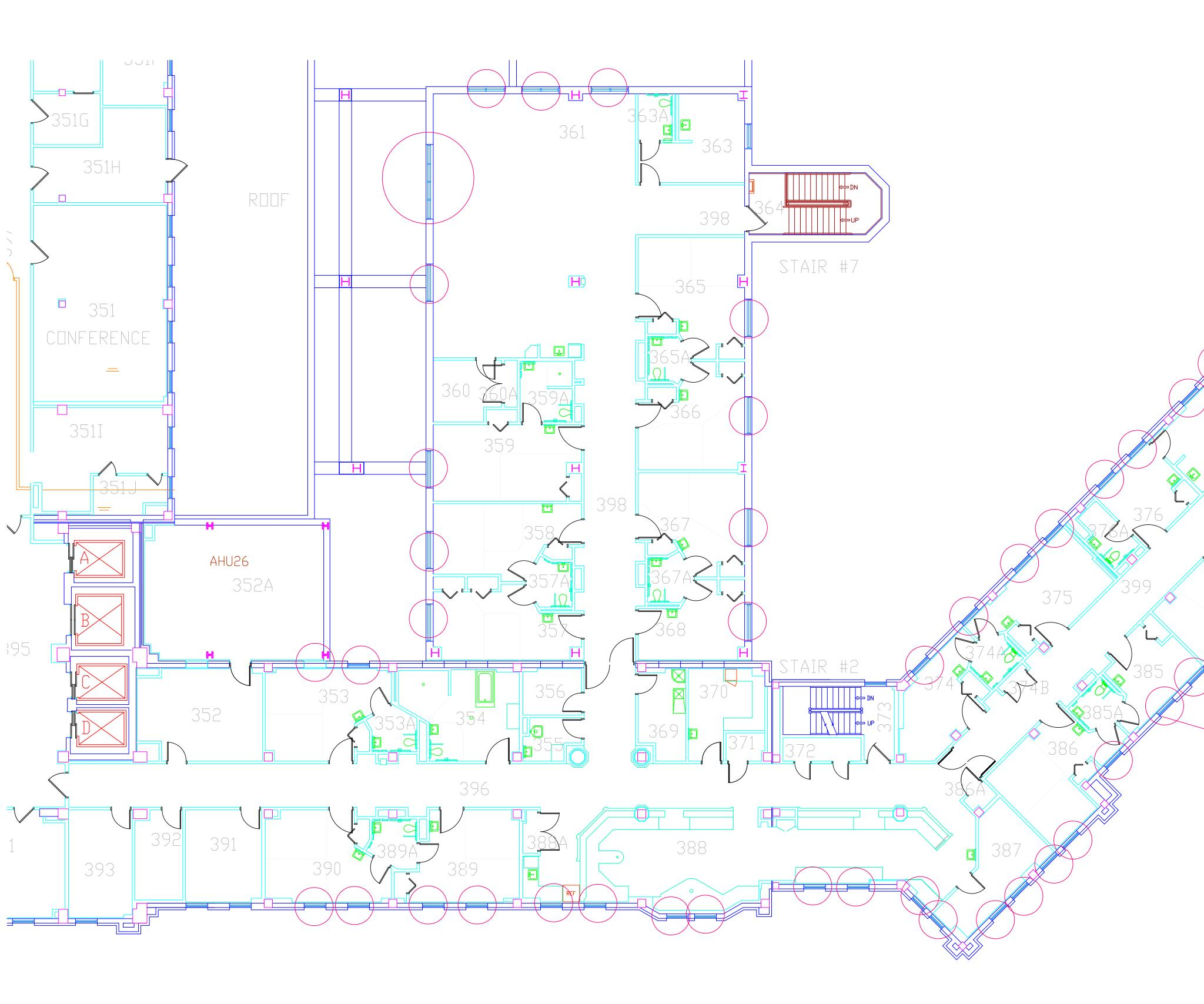
Contractor shall demolish all existing window coverings and window sills circled in pink and replace with new window sills and window coverings as indicated in finish schedule. Contractor to repair any wall damage as a result of removing window sill. Contractor is required to field verify all window covering and window sill measurements prior to ordering and installation.
